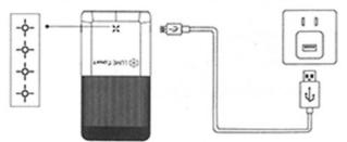
\*To preserve battery lifespan, use and recharge at least once every 4 months. When your power bank is fully charged, the LED indicators will fully light up and stop blinking. To give your power bank fastest, safest recharge, use an original LUME-16 smart high-speed power or an other certified adapter.
